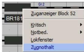
This menu shows the menu items of a block. As an extra, a locomotive window can be opened to operate the locomotive that is currently in the block, and the train can be stopped in the block (train emergency stop).
