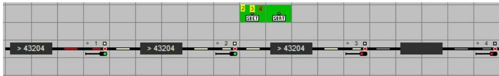
If the route from Signal 1 to Signal 2 has entered and is set, the occupancy of the 1st block section through the active SSB / aSB also the route from signal 2 to 3.
