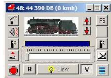
When the locomotive window is active, the speed can alternatively be set with the cursor keys ( / ) or can be changed with the mouse wheel.
